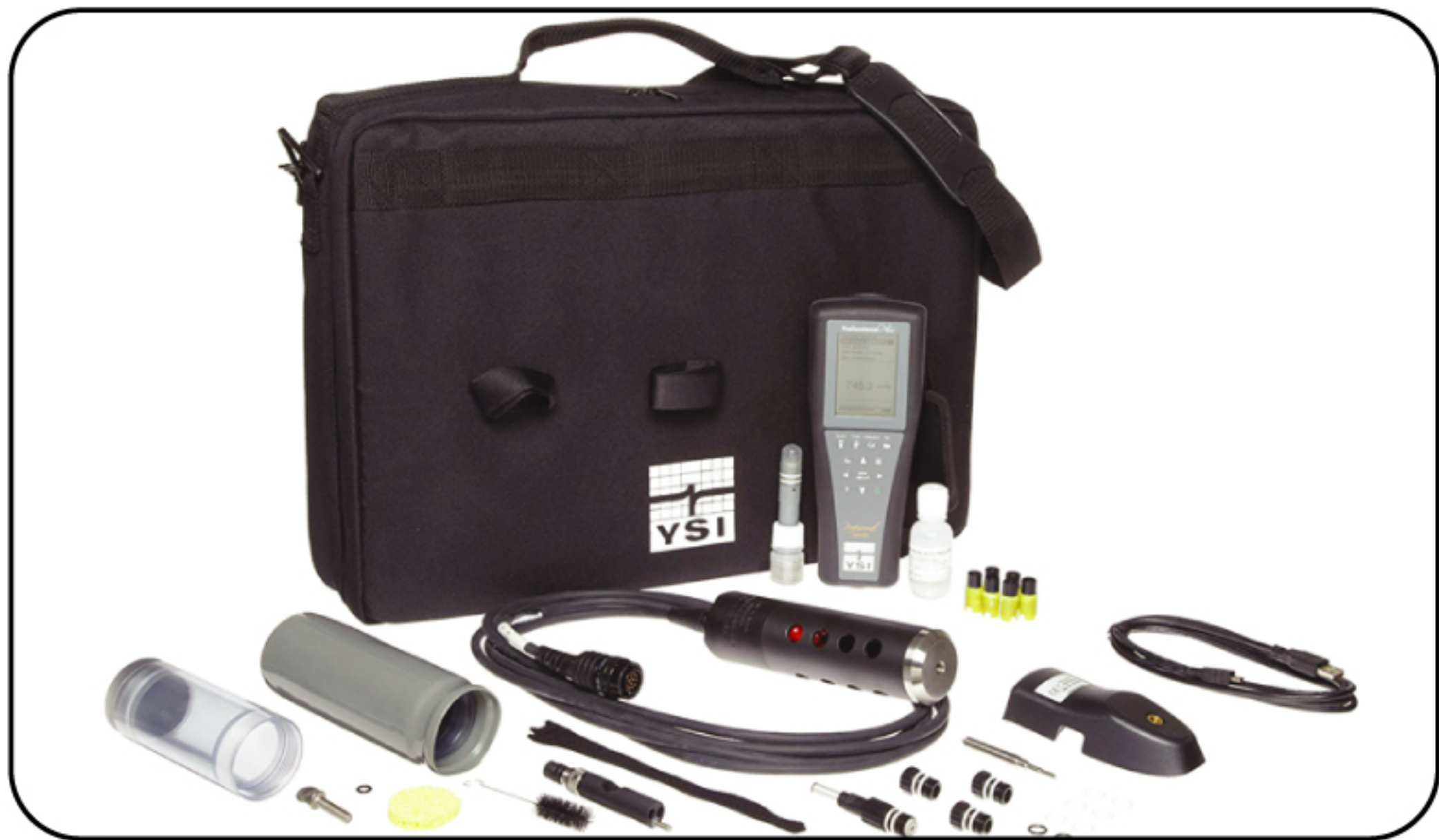
Multi-Parameter Water quality measuring meter
