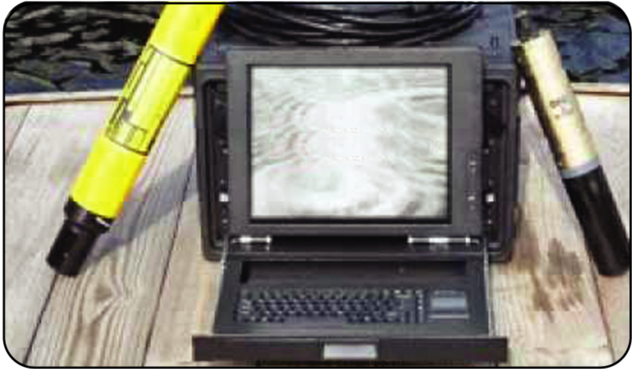
Side Scan Sonar - Edgetech 4125
